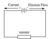
• When a battery is not connected to any circuit, the potential difference across the terminals of the battery is equal to the EMF of the battery. (EMF = Electro Motive Force).
